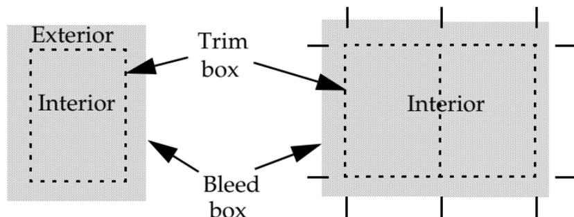
The interior and exterior are enclosed by (usually invisible) boxes called the *trim box* and the *bleed box*. If the trim box and bleed box are the same, there is no bleed exterior at all, and the page is said to have no bleed defined.
