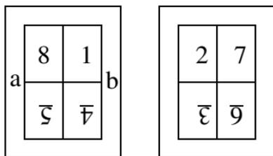
This sheet would be printed on both sides, folded along the line *a* to *b* first, then the final fold.
